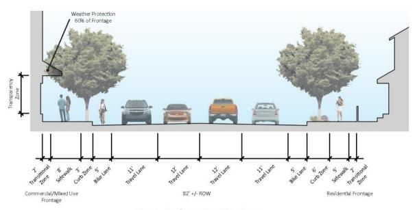
Figure 10-3. Commercial Mixed Use Belfair Street Section
