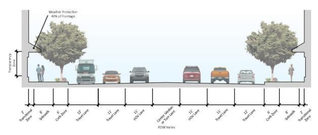
**Figure 10-5. Commercial Corridor Street Section**
