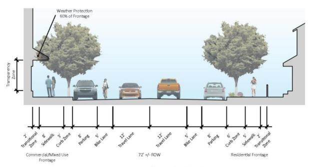
Figure 10-2. Commercial Mixed Use Street Section
