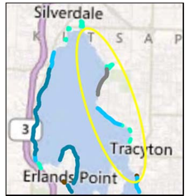
Sediment source mapping delineated a shallow landslide reach (blue) and a deep-seated landslide reach (gray), as well as four tributaries (green)
