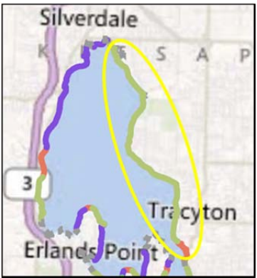
Net shore drift showing right-to-left sediment transport (in this case, from south to north) in drift cell
