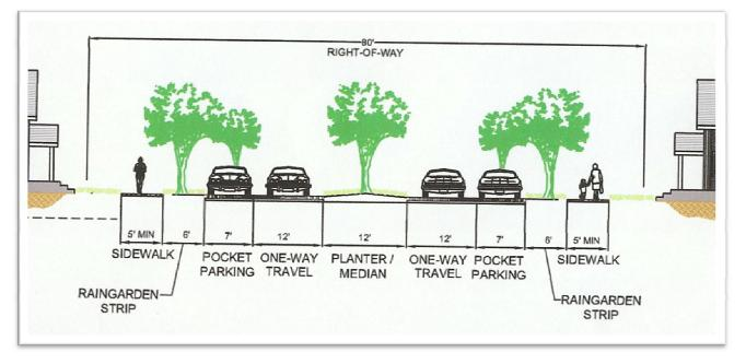
Figure 15.4: Example of "parkway" with narrow travel lanes and pocket parking with sidewalk separated by raingarden/bioretention strip for appeal, safety and stormwater sheet flow to facility.
