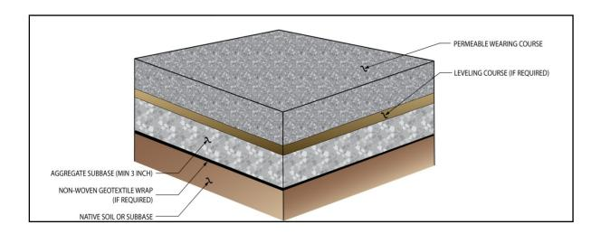
Figure 1.2: Typical Permeable Pavement Surface Section Source: City of Seattle Stormwater Flow Control and Water Quality Treatment Technical Requirements Manual
