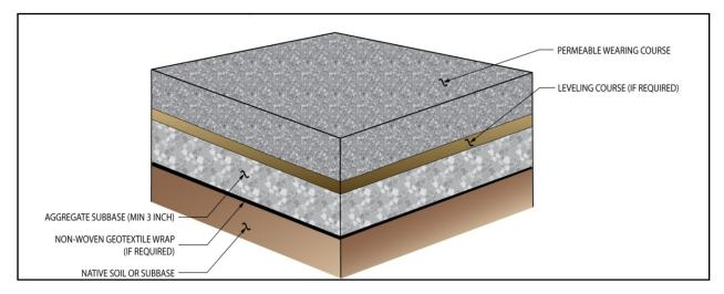
Figure 2.1: Typical Permeable Pavement Surface Section Source: City of Seattle Stormwater Flow Control and Water Quality Treatment Technical Requirements Manual
