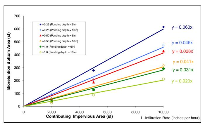
Figure C6. Bioretention facility (bottom area) sized for water quality treatment as a function of contributing impervious area (annual precipitation of 36 inches).
