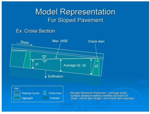
*Figure2.3: Modeling representation of sloped base storage with check dams Source: Herrera Environmental Consultants*
