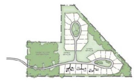
Figure 12.1: A large lot conservation design for protecting open space that uses shared driveways to access homes.
