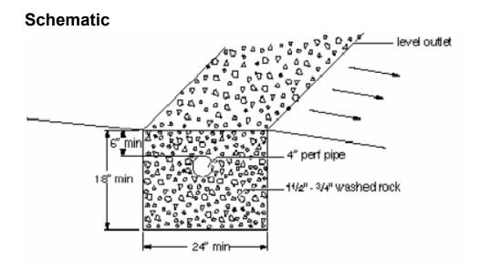
Figure 5.1: Cross section of typical level spreader trench for infiltrating and/or dispersing stormflows across a slope. Note the level outlet at the down-gradient lip of the trench to prevent concentrated flows.(From SMMWW Vol 5)
