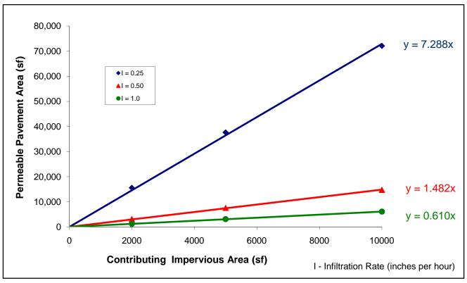
Figure C12. Permeable pavement facility sized for flow control as a function of contributing impervious area (annual precipitation of 52 inches).
