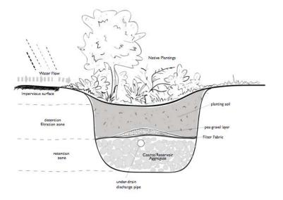
Figure 9.2: Bioretention cell or raingarden with underdrain – typically used where slower infiltration rates or space constraints prevent the sizing of facilities to manage peak design flows. Drain is elevated above bottom of cell to allow full infiltration of typical events, with overflow relief for larger events.
