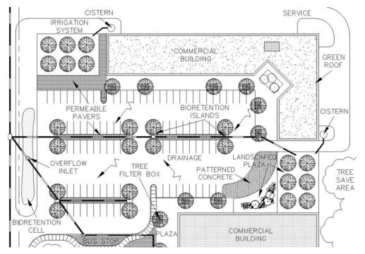
Figure 18.1: Example of layout of commercial hardscape with planters, tree containers and bioretention islands to manage stormwater runoff from impervious paving.
