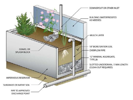
Fig. 18.2: Typical cross-section of a bioretention planter (City of Seattle)
