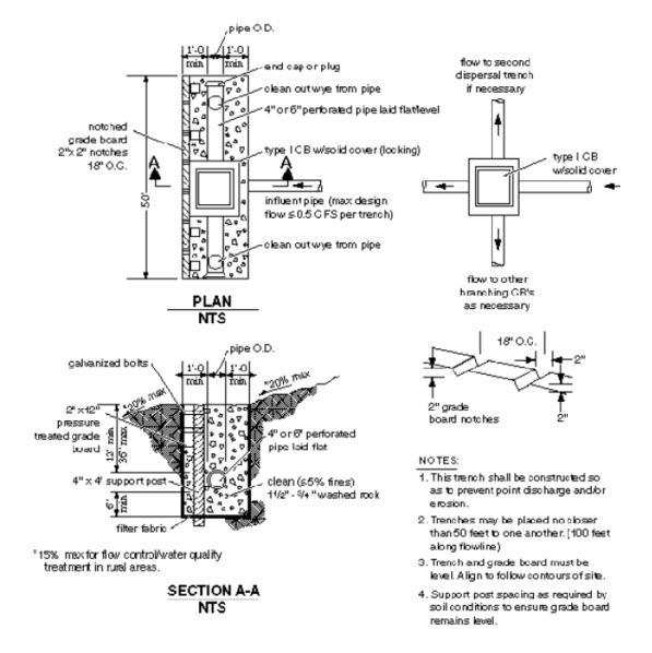
*Figure 5.2:* Details of a standard dispersion trench with a notched grade board for dispersing concentrated stormflows across a slope.
