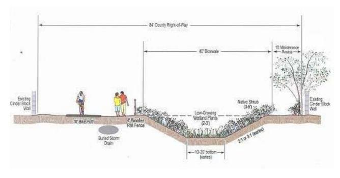
Figure 9.3: Cross section of a linear bioretention cell or swale – allowing for 100% infiltration or evaporation of inflowing stormwater
