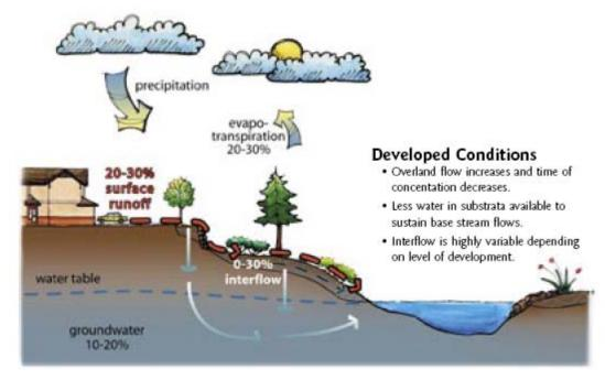
*Fig* 3 – *Hydrological cycle for conventionally developed conditions in Puget Sound. Source:* LID Technical Guidance Manual 2005
