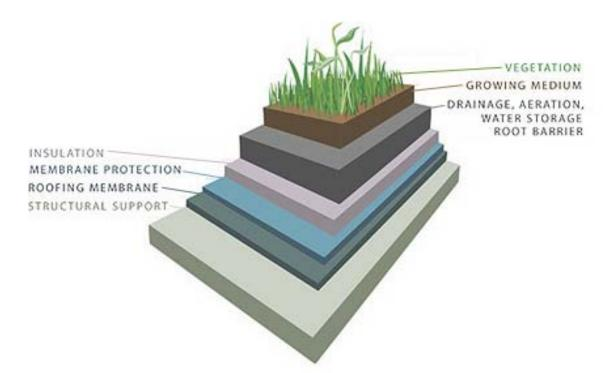
Figure 7.2: Typical built-up vegetated roof system assembly. Source: NA
