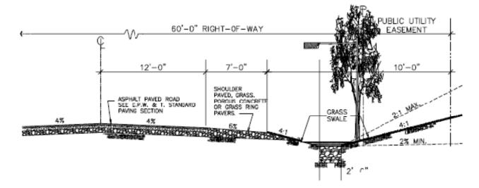
Figure 15.3: A rural residential right-of-way section has the same 60-foot width, but reduces paving width by 33% to 24 feet, and eliminates the use of concrete curb and gutter
