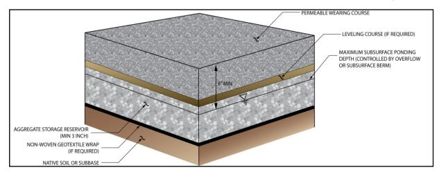
Figure 1.3: Typical Permeable Pavement Facility Section - (Maximum ponding depth kept to a minimum of 6" below the surface of the wearing course to prevent saturation of wearing course and possible freeze/thaw damage)
