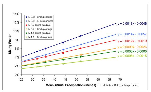
Figure 5. Bioretention water quality sizing factors for Kitsap County as a function of mean annual precipitation.
