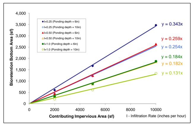
Figure C3. Bioretention facility (bottom area) sized for flow control as a function of contributing impervious area (annual precipitation of 44 inches).
