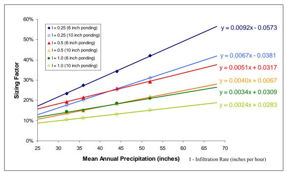
Figure 4. Bioretention flow control sizing factors for Kitsap County as a function of mean annual precipitation.
