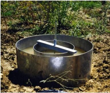
Examples of Double Ring Infiltrometers.
