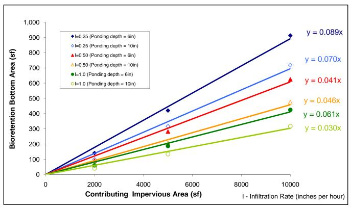
Figure C8. Bioretention facility (bottom area) sized for water quality treatment as a function of contributing impervious area (annual precipitation of 52 inches).
