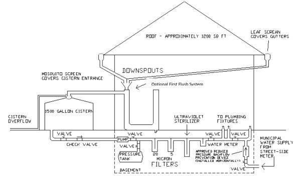
Figure 8.1: Typical Roofwater harvesting system. Source: Experiments in Sustainable Living
