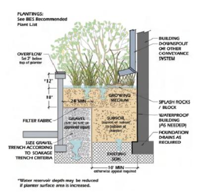
Figure 18.3: Typical cross-section of an infiltration planter – representation not for design purposes (City of Portland)
