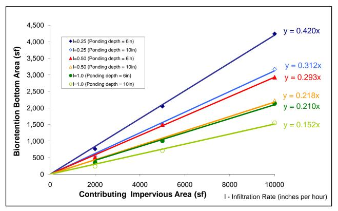
Figure C4. Bioretention facility (bottom area) sized for flow control as a function of contributing impervious area (annual precipitation of 52 inches).
