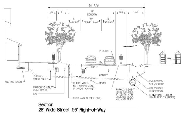
Figure 15.3: Section from High Point, West Seattle, showing electric utility vault location
