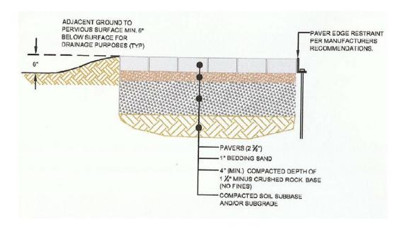
Figure 4.1: Typical Pervious Paver section for sidewalk or patio. Vehicle bearing installations would typically have thicker base courses. Source: 2020 Engineering 2008
