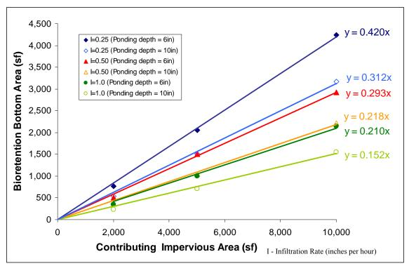
Figure 2. Bioretention facility (bottom area) sized for flow control as a function of contributing impervious area (mean annual precipitation of 52 inches).
