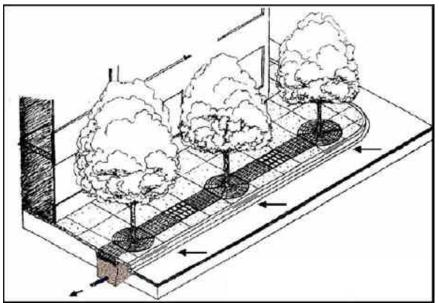
Figure 18.4: Manufactured Tree Box Filters For Stormwater Management (Source: Low Impact Development Center)
