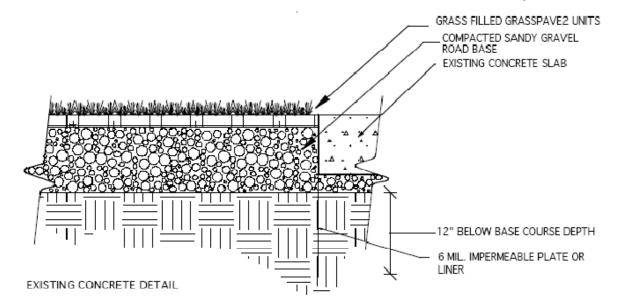
Figure 3.3: Typical section for cellular reinforced grass pavement adjacent to conventional impervious pavement. Source: NA
