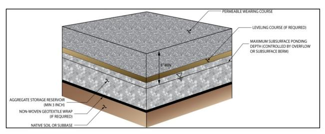
Figure 2.2: Typical Permeable Pavement Facility Section – (Maximum ponding depth kept to a minimum of 6" below the surface of the wearing course to prevent saturation of wearing course and possible freeze/thaw damage)
