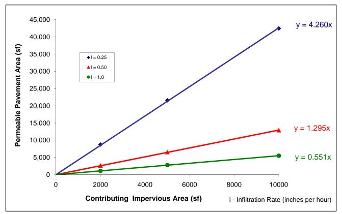
Figure C11. Permeable pavement facility sized for flow control as a function of contributing impervious area (annual precipitation of 44 inches).
