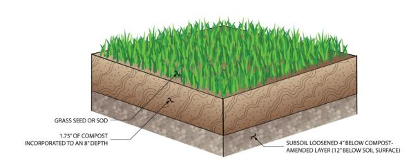
Figure 6.2: Cross Section of Turf Soil Amendment. (Source: Seattle Public Utilities/Seattle Department of Planning and Development)
