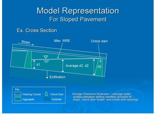
*Figure 4.3: Modeling representation of sloped base storage with check dams Source: Herrera Environmental Consultants*
