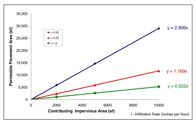
Figure C10. Permeable pavement facility sized for flow control as a function of contributing impervious area (annual precipitation of 36 inches).
