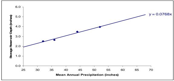
Figure 7. Permeable pavement surface depth for Kitsap County as a function of mean annual precipitation (for installations at up to 2 percent slope).
