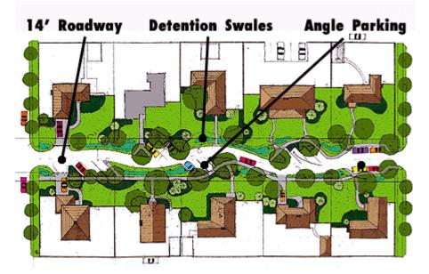
Figure 14.1: Schematic of a section of the SEAStreets Layout. Source: Seattle Public Utilities
