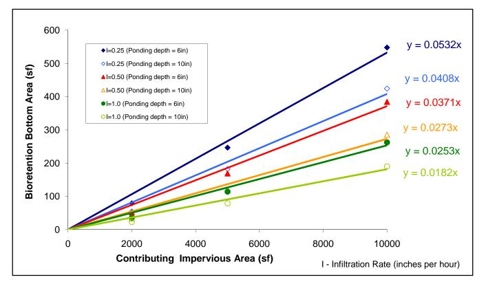
Figure C5. Bioretention facility (bottom area) sized for water quality treatment as a function of contributing impervious area (annual precipitation of 32 inches).
