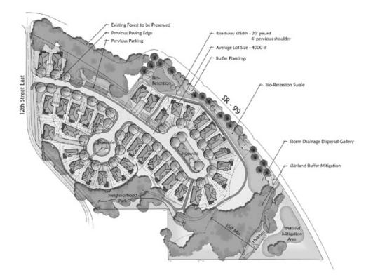
Figure 17.1: Meadow on the Hylebos site plan (LID Technical Guidance Manual2005)
