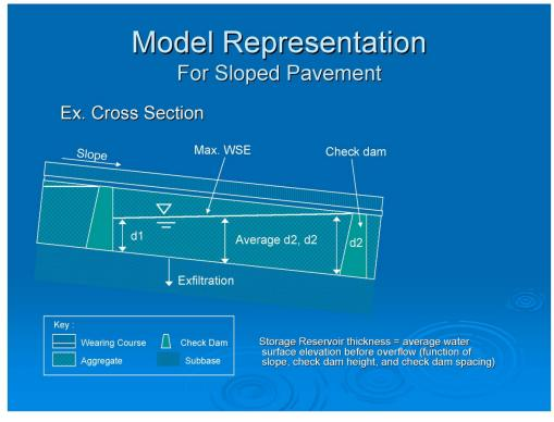
*Figure 3.4: Modeling representation of sloped base storage with check dams Source: Herrera Environmental Consultants*
