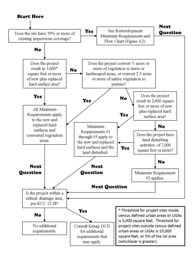
Figure 4.1 – Flow Chart for Determining Minimum Requirements for New Development Projects
