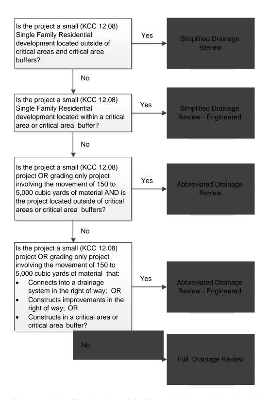
Figure 1.1 – Flow Chart for Determining Type of Drainage Review Required
