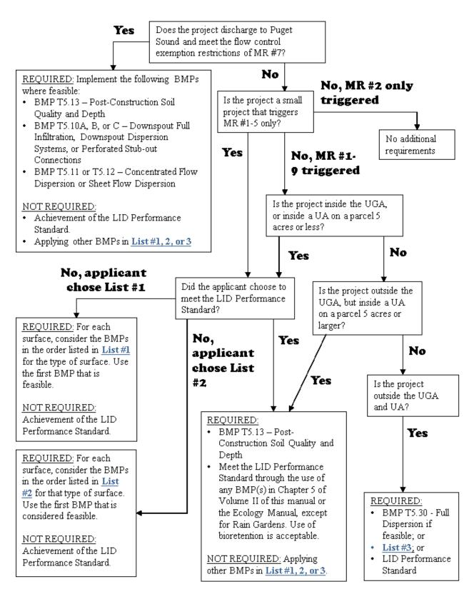
Figure 4.3 – Flow Chart for Determining LID MR #5 Requirements
