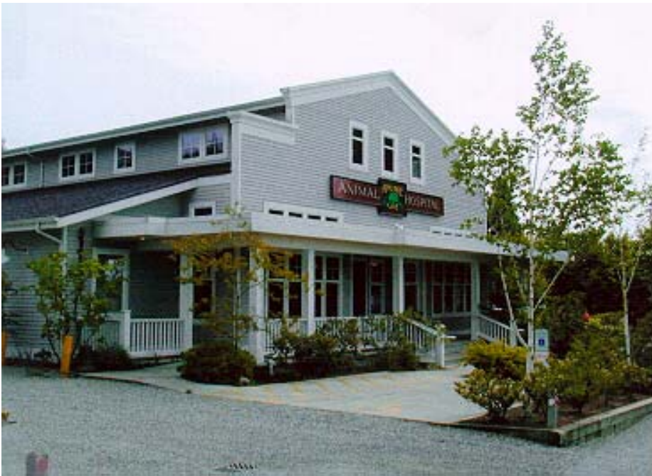
Figure IV-2. This contemporary interpretation of traditional architecture would be appropriate in all three downtown districts. The simple gable form, traditional siding, appropriate sign, welcoming porch, and "transparent" front façade make it pedestrian friendly and consistent with the town's identity. Note how the multi-paned windows, porch railing, and porch column details all add a simple grace and human scale without being overly ornamental. The colors, light gray with white trim, are appropriate. The landscaping also enhances the development's qualities.
