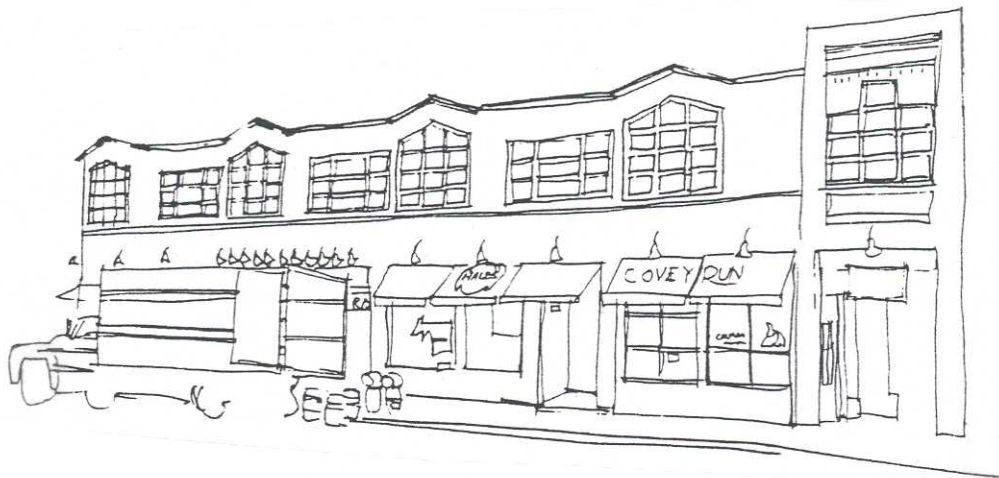
Figure IV.C.1.(c). The roofline, windows, and details of these examples are coordinated to provide a rhythmic breakup of an otherwise horizontal building. Note how the awnings and lights provide human scale while their repetition relates back to the building massing.
