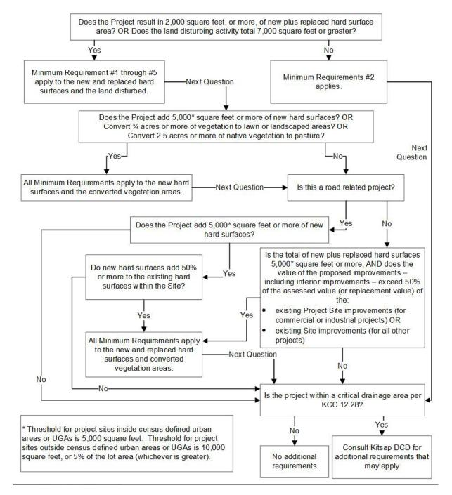
Figure <u>I-4.12.4.1</u> – Flow Chart for Determining Requirements for New Development
