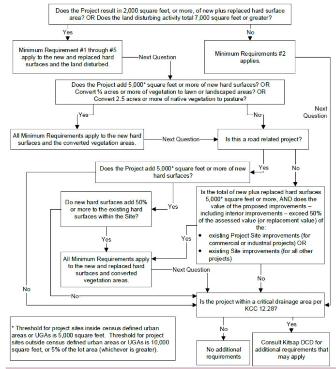
Figure <u>I-4.22.4.2</u> – Flow Chart for Determining Requirements for Redevelopment
