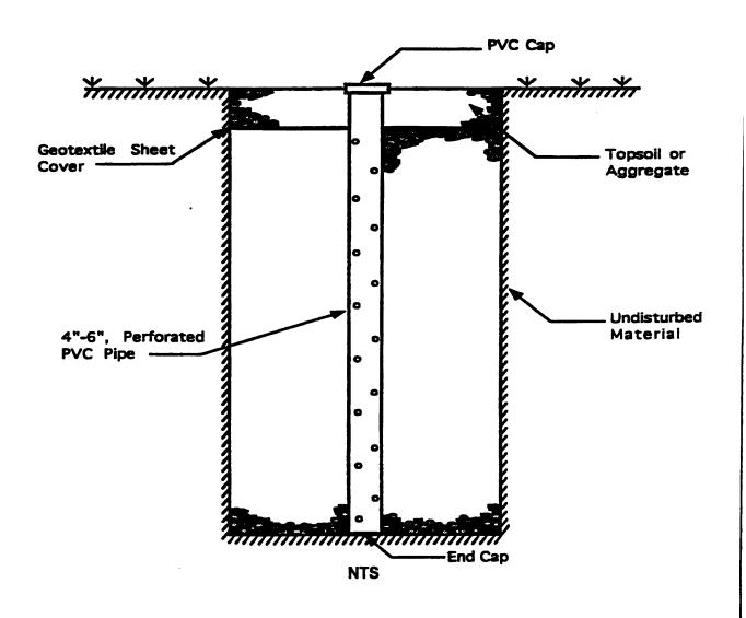
Figure 5-25 INDIVIDUAL DOWNSPOUT INFILTRATION SYSTEM Roof Roof Drain Trench PLAN VIEW Not to Scale Roof Observational Well (Optional) 4" Perforated Pipe Sump w/ Solid Lid Roof Drain PROFILE VIEW nts Overflow GeotextileSheet Splash Block Cover\_ SECTION A-A Not to Scale
