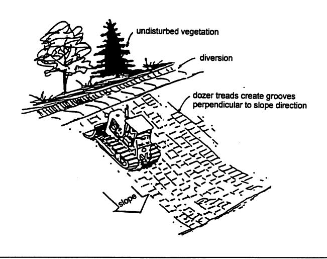
Figure 3-4 STAIR-STEPPING CUT SLOPES AND GROOVING SLOPES
