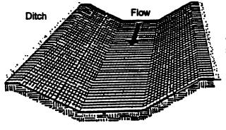
In ditches, apply netting parallel to the direction of flow. Use check slots every 15 feet. Do not join strips in the center of the ditch.
