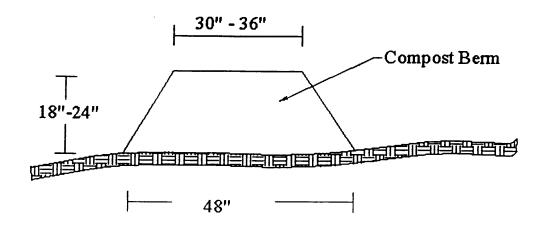
Compost Berm Steep Slope (5-10%) Applications (Not to Scale)
