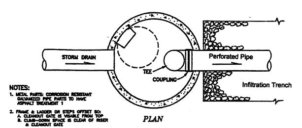
3. IF METAL OUTLET PIPE CONNECTS TO CEMENT CONCRETE PIPE: OUTLET PIPE TO HAVE SMOOTH O.D. EQUAL TO CONCRETE PIPE LD. LESS  $1/\mathcal{C}$
