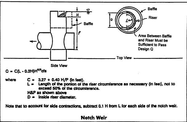
6. Properly designed weirs, such as rectangular notched weirs, v-notched weirs, or sutro weirs, may be used as flow restrictors located either in catch basin structures, or mounted on a concrete retaining structure in the open. Formulas for sizing rectangular notched weirs and v-notched weirs are as follows:
