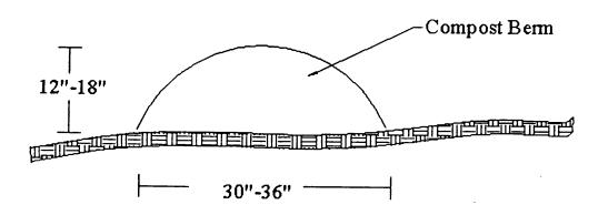
Compost Berm Shallow Slope (<5%) Applications (Not to Scale)
