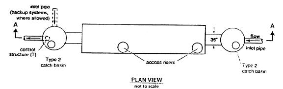
"Flow through" system shown solid Designs for "flow backup" system and parallel tanks shown dashed
