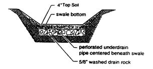
NOTE: Underdrain must infiltrate or drain freely to an acceptable discharge point.
