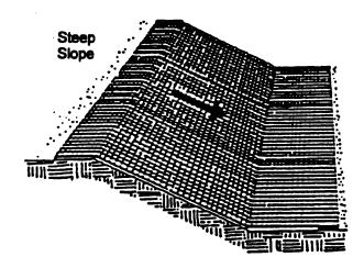
On steep slopes, apply strips of netting parallel to the direction of flow and anchor securely. (Slopes greater than 1:1)
