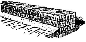
Construction of A Straw Bale Barrier
