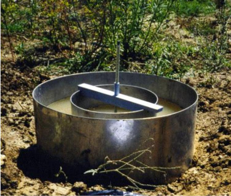
Examples of Double Ring Infiltrimeters.
