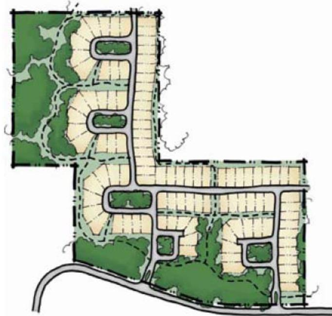
Figure 13.1: An open space layout showing decreased pavement area and common stormwater infiltration areas.
