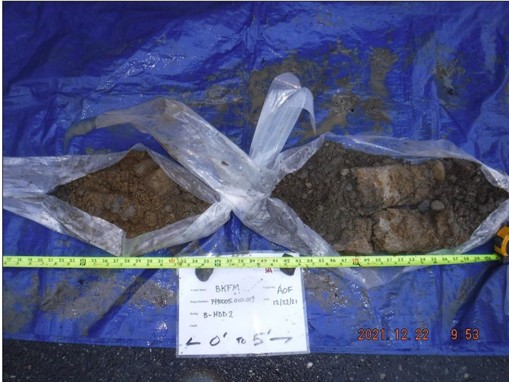
17. Boring B-HDD2, 0 to 5 feet deep.
