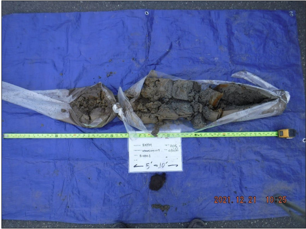
3. Boring B-HDD1, 5 to 10 feet deep.
