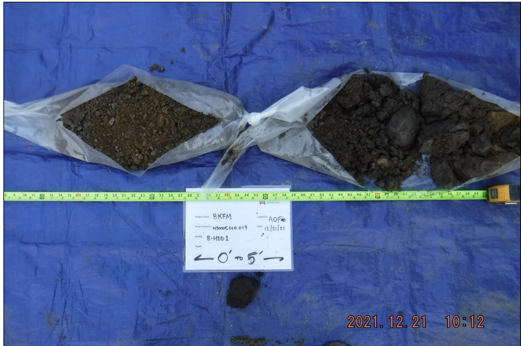
1. Boring B-HDD1, 0 to 5 feet deep.
